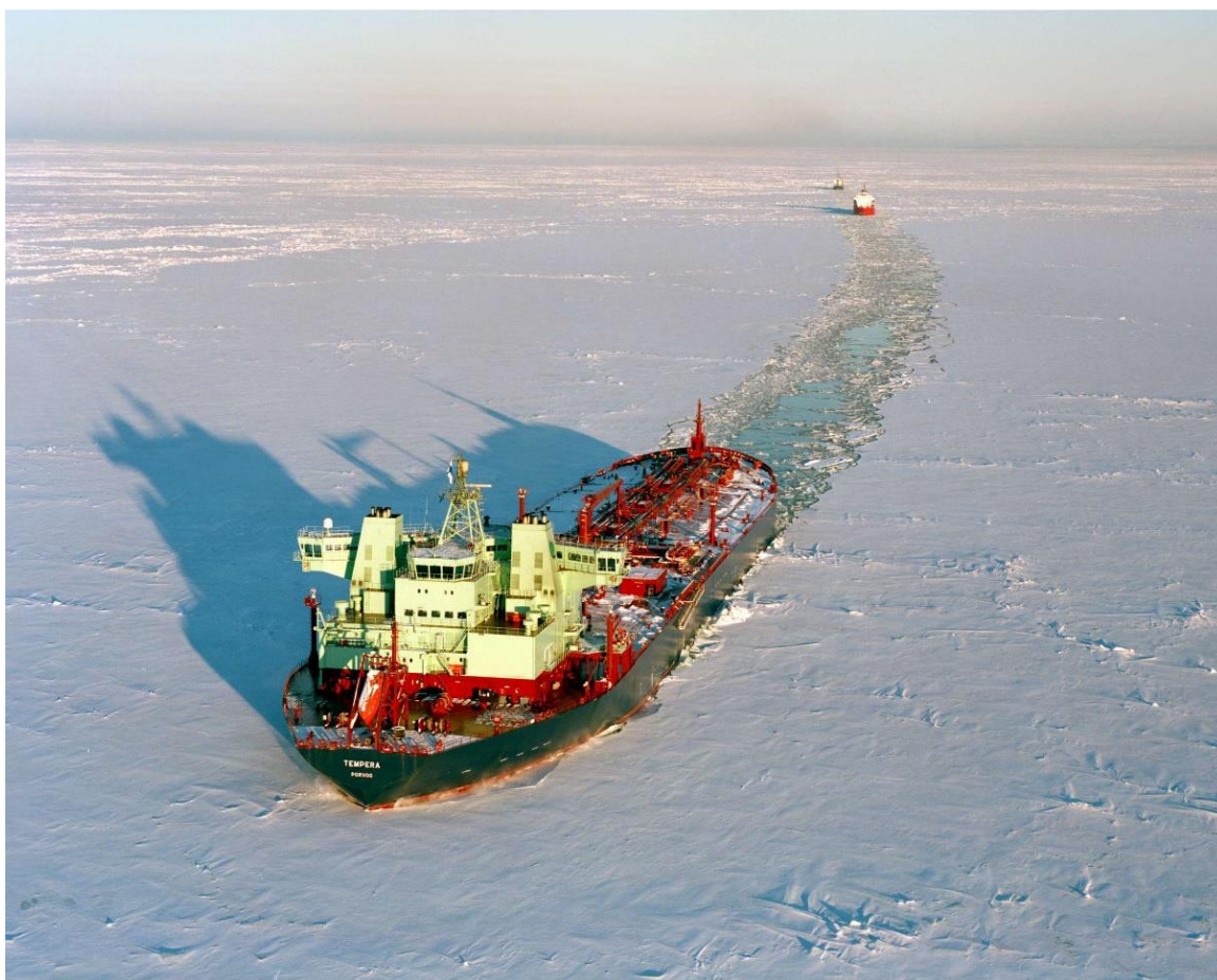
Figure 46. Double acting tanker Tempera moving astern in the ice conditions of Gulf of Finland
