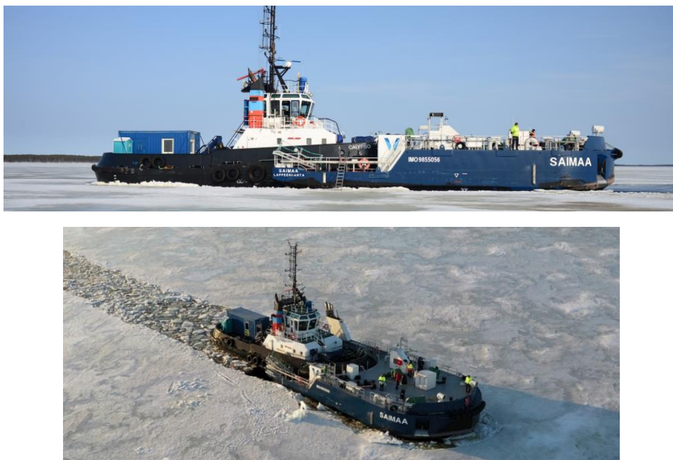
Figure 51. Detachable icebreaking bow Saimaa (blue) attached to tug Calypso (black).
