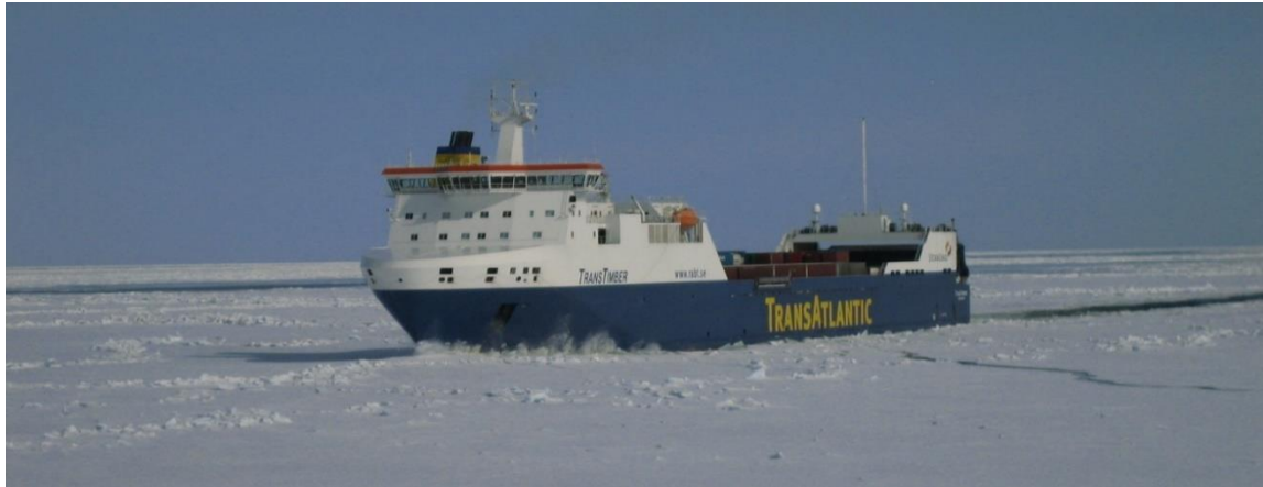
Figure 45. IA Super ice class ferry with bulbous bow in independent operation in ice
