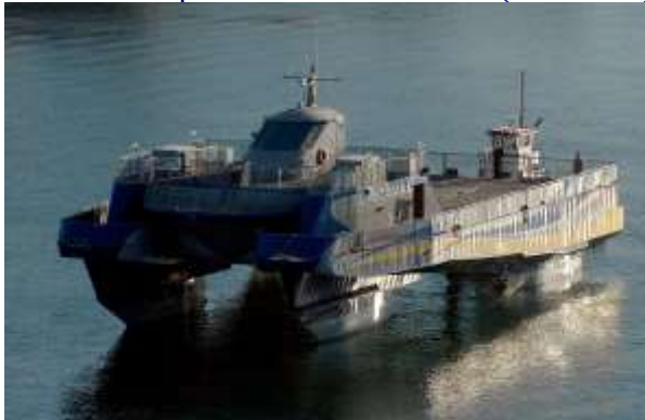
Small Waterplane Area Multi-Hull (SWAMH)
