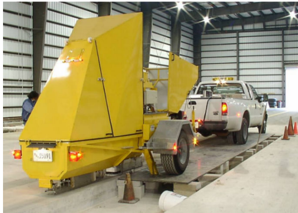
Foto 3.1. KUABi põhiseade ehk kahemassiline FWD. Foto allikast: U.S Department of Transportation. Federal Aviation Administration, [5]
