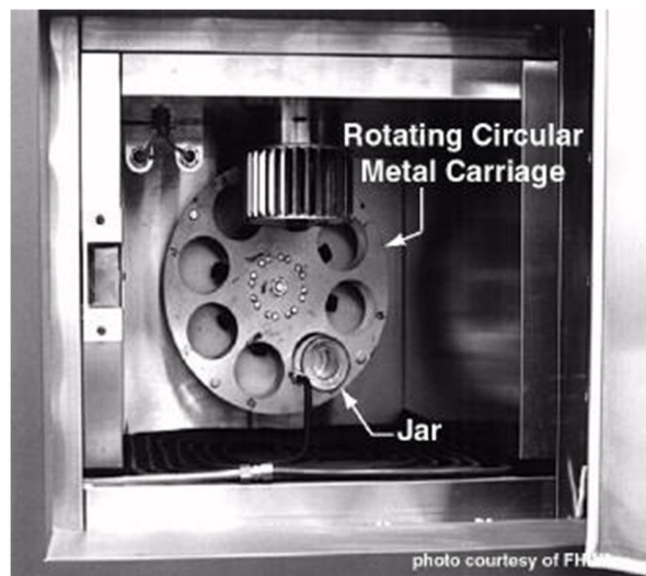
Joonis 4.1. Rolling Thin Film Oven [Pavementinteractive]
