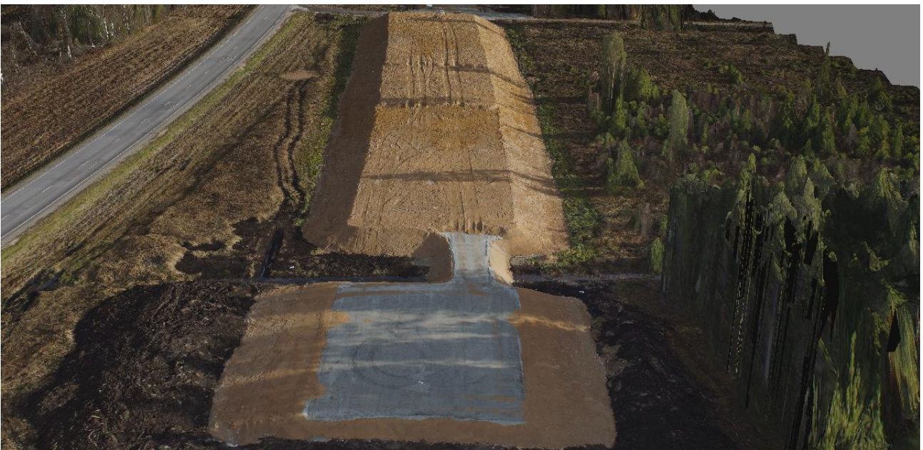
Figure 13. 3D surface model created from the RPAS photos combined with aerial photos (Julge 2015). Surface after construction of surcharge loading 5.11.2015 (RPAS=Remotely Piloted Aircraft System).
