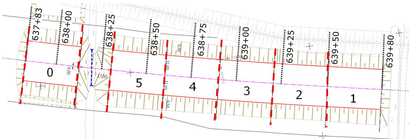
Figure 3. Test sections. 0. mass replacement, 1. one layer and 2. two layers of georeinforcements, 3. geocell mattress, 4. light weight aggregate and 5. EPS light weight embankment structure. Tallinn is on the left.
