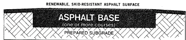
Skeem 1. Paks asfaltkate - full-depth asphalt pavement
