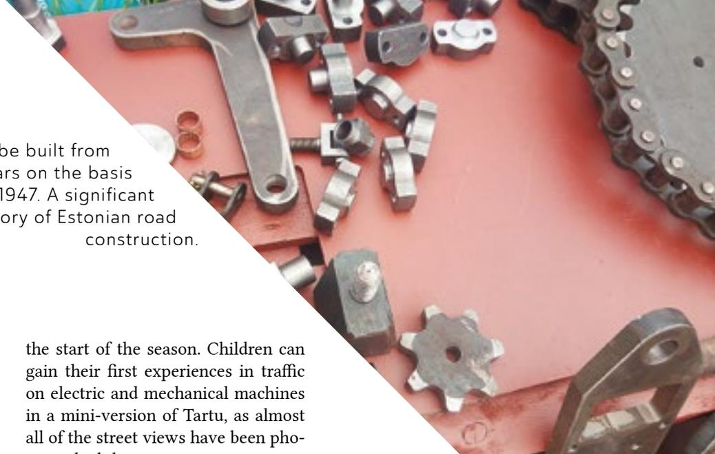
The V-1 road grader will be built from these parts in three years on the basis of drawings dating from 1947. A significant machine in the history of Estonian road construction.
